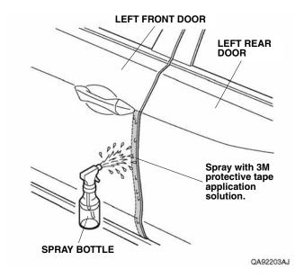
If the vehicle is equipped with the door lower trim, go to step 5.
