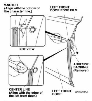
4. Align the center line on the left front door edge film with the edge of the left front door. While applying light pressure, carefully remove the adhesive backing, and attach the left front door edge film to the left front door. Go to step 8.
