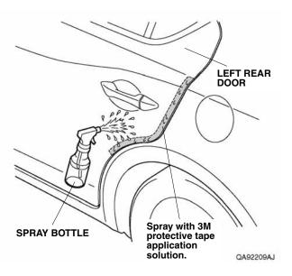
13. Open the left rear door. Peel back about 50 mm (2.0 in.) of adhesive backing from the left rear door edge film. Align the V-notch 30 mm (1.2 in.) above the character line on the upper part of the left rear door as shown.
