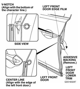
7. Align the center line on the left front door edge film with the edge of the left front door. While applying light pressure, carefully remove the adhesive backing, and attach the left front door edge film to the left front door.
