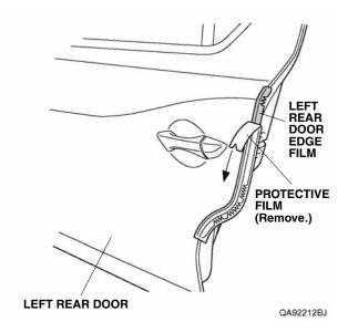
17. Starting from the center and working outward, use your fingers to fold the left rear door edge film around the edge of the left rear door. Move your fingers in one direction. Attach the left rear door edge film over the seam sealant. Do not trim or damage the seam sealant.
