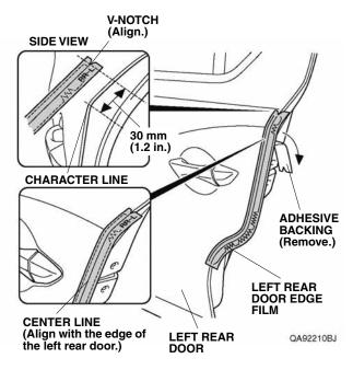
14. Align the center line on the left rear door edge film with the edge of the left rear door. While applying light pressure, carefully remove the adhesive backing, and attach the left rear door edge film to the left rear door.  Starting from the top and working downward, use the soft sleeve to smooth the left rear door edge film. Move the soft sleeve in one direction only.
