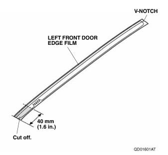
6. Open the left front door. Peel back about 50 mm (2.0 in.) of adhesive backing from the left front door edge film. Align the V-notch with the bottom of the character line on the left front door as shown.
