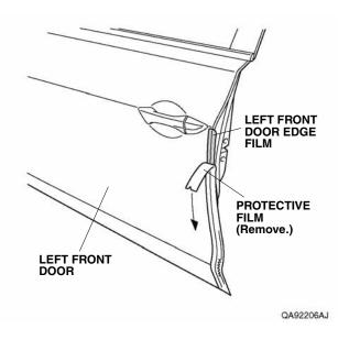
10. Starting from the center and working outward, use your fingers to fold the left front door edge film around the edge of the left front door. Move your fingers in one direction. Attach the left front door edge film over the seam sealant. Do not trim or damage the seam sealant.
