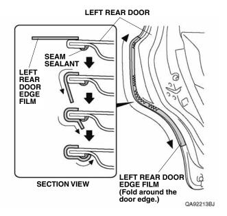
18. Using a shop towel, wipe the 3M Protective Tape Application Solution from the left rear door edge film. Allow the left rear door edge film to dry thoroughly.
