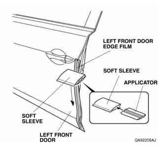
9. Slowly remove the protective film from the left front door edge film.
